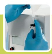
Site tube on the front of the unit allows for **quick indication of the fluid level**
